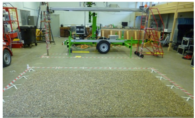
Figure 1. The GB-SAR system set up indoors with a gravel scene to be imaged. The X-band antenna horns are mounted on a SAR rail, which is mounted on the Green "Niftylift120" trailer. Metal spheres, with both 3cm and 5cm diameter are setup on either side (left and right) to aid in image alignment and resolution estimation.
