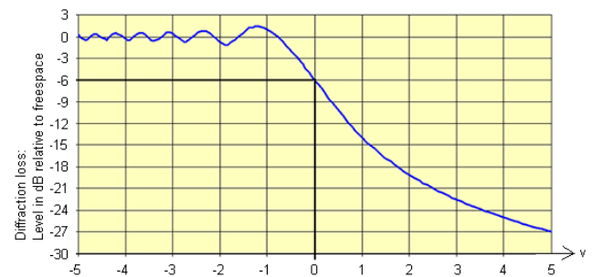
Figure 4. Diffraction loss of a "knife-edge" versus parameter v [4]
