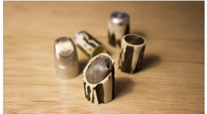
Figure 1. Sketch (a) above showing the design of the thimble consisting of two essential parts, a rigid cylindrical base, and a thin conductive fabric for the finger tip. Photo (b) below showing a number of thimbles resulting from exploring suitable materials, with the front thimble showing a rigid base made from antler combined with a grey conductive fabric tip.
