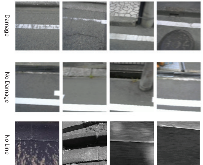
Figure 2. Dataset samples. Each image is 224 \times 224 pixels by random clipping from video frames, respectively. The images at top row show damaged line, the images at mid row undamaged and at bottom row no line.
