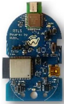
Figure 4. Wearable device prototype of the GuideMe project.
