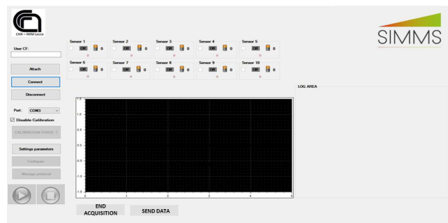
Figure 2. Interface of the software developed for the acquisition of raw EMG signals, data elaboration and sending to external processes.
