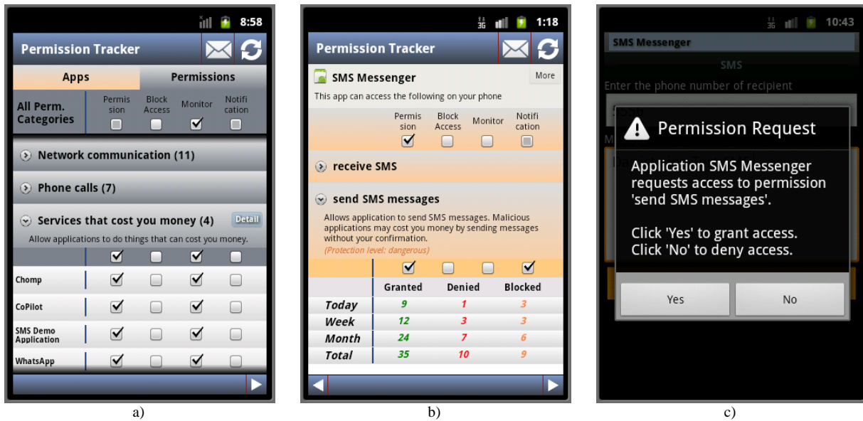
Figure 4. a) PermissionTracker showing permissions' applications. b) Granted, denied and blocked permissions. c) Permission request
