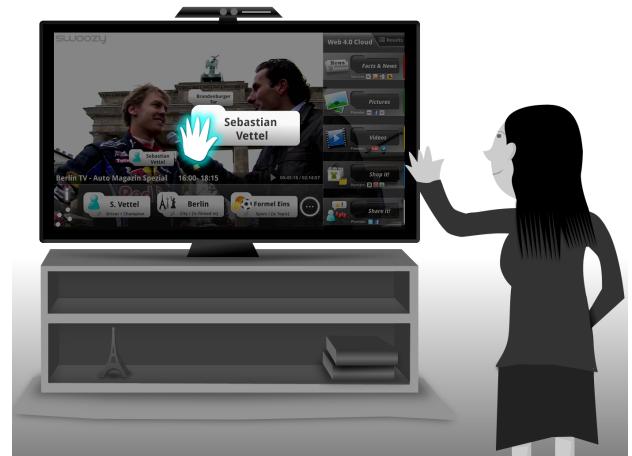
Figure 8. User gesture interaction: a virtual hand allows the user to grab out a semantic term from a video.
