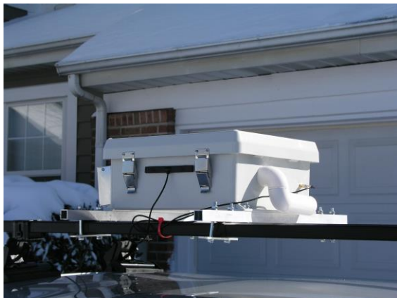
Figure 2. Public transportation sensor mounted on a car for experimentation.
