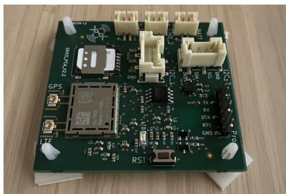
Figure 1. The OKKO board: ESP32-S2 microcontroller + HL7800 LTE-M modem + I2C connectors.
