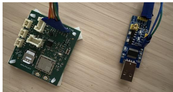
Figure 2. Assembly for uploading Arduino code to the OKKO board.
