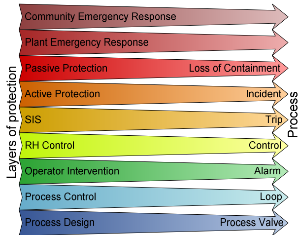
Figure 2 - Layers of protection and impact on process
