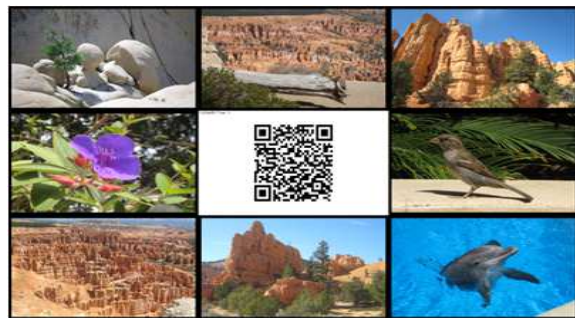
Figure 6. Video frame identification and clock synchronization by QR Code insertion/decoding.
