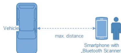
Figure 2. Test arrangement for the detection of Secondary Vehicle Identifier in stand still mode
