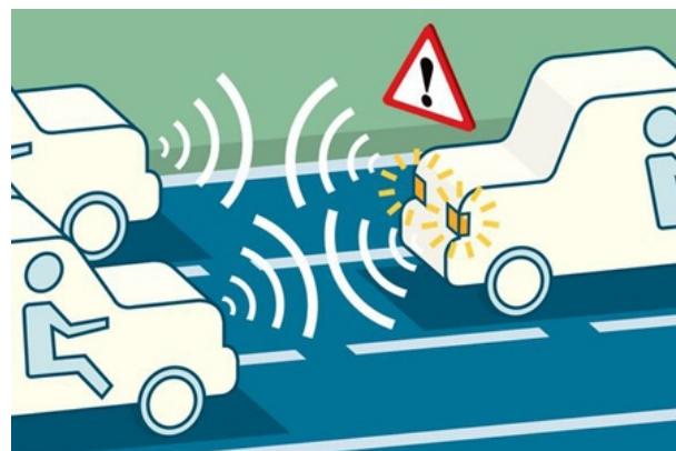
Figure 1. Visible Light Communication for V2V information exchange.
