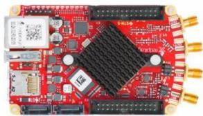
Figure 5. Red Pitaya hardware, which provides the backend for generating and recording CAN signals
