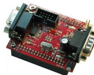
Figure 9. AT90CAN128 development board used to generate CAN messages [10]
