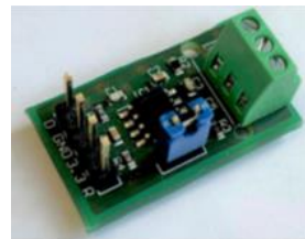
Figure 7. Circuit board of the VP230 on the server side
