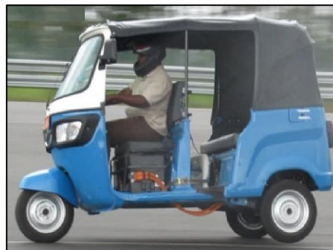
Figure 12. Constant Radius Cornering at Test rack.
