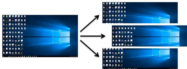
Figure 5. OCR capture process, splitting fullscreen images into 2n - 1 slices for executing overlapping subtasks in parallel threads to reduce OCR execution time.
