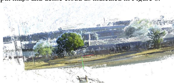
Figure 8. Denser point of cloud with multiview stereo.
