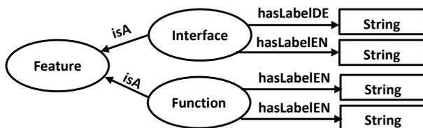
Figure 2. Structure of the software feature ontology
