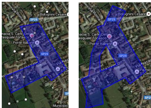
Figure 3. Drawing overlapping polygons. On the left: an existing polygon (in blue) and a new area, delimited by its corners (white dots). On the right: the result of polygon union.
