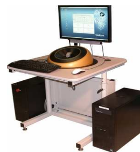
Figure 2. Maglev 200 ™ Magnetic Levitation Haptics
