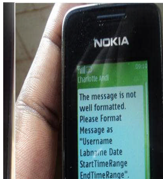
Figure 8. System response to a wrongly formatted message
