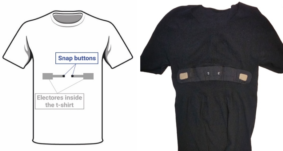
Figure 1. The smart t-shirt schema and a photo of the prototype.
