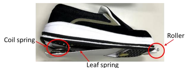
Figure 6. Heel-assist shoe prototype.
