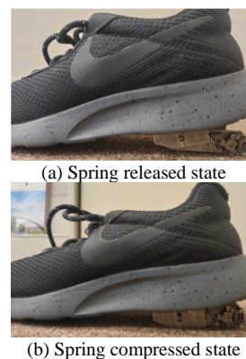
Figure 11. Pair of shoes incorporating the evolved heel-raising unit.
